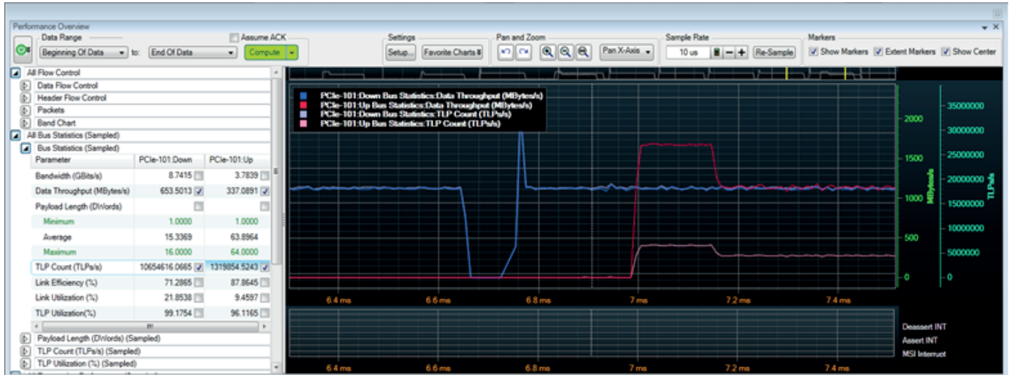
Figure 15. The statistical performance of the link latency, utilization, and Flow Control credits, is shown with events such as Interrupts and errors.
